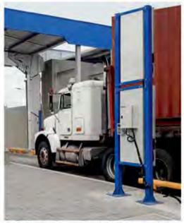
The photo shows an example of Vehicle Radiation Monitor
